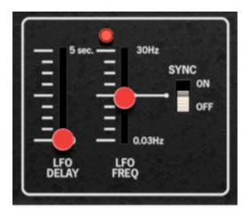
The LFO (low-frequency oscillator ) generates sub-audio range signals intended for modulation purposes.
