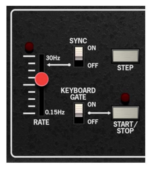
**Rate**- Sets the overall speed of the sequencer clock, i.e. how fast it moves from step to step, from 0.15 to 30 Hz. The indicator lamp above the slider displays the current tempo.
