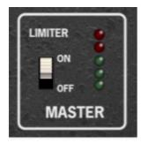
**Limiter**- The *Limiter* switch applies a transparent limiting effect to help prevent overloading. This is particularly useful with higher *Number of Voices* settings.
