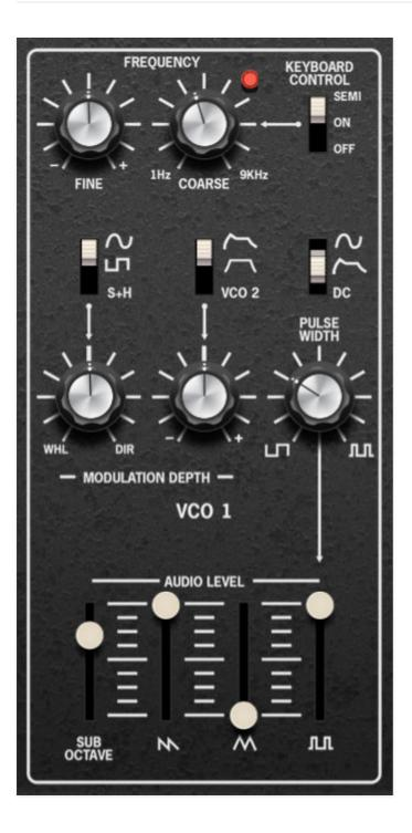
**Fine Tune**- This can be used to fatten dual oscillator patches by detuning a small amount, or for "building-in" musical intervals. Its range is a roughly a minor third, up or down.
