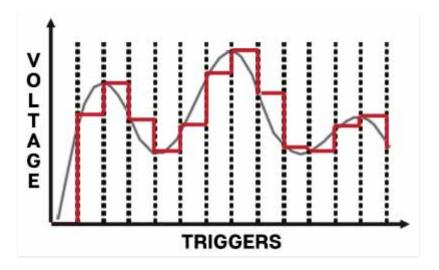
White noise is often used as an input source to generate a random stepped-CV signal. Modulating the pitch of an oscillator with this will create the classic sample and hold sound often heard in sci-fi movies, perhaps most recognizably as the voice of R2-D2.
