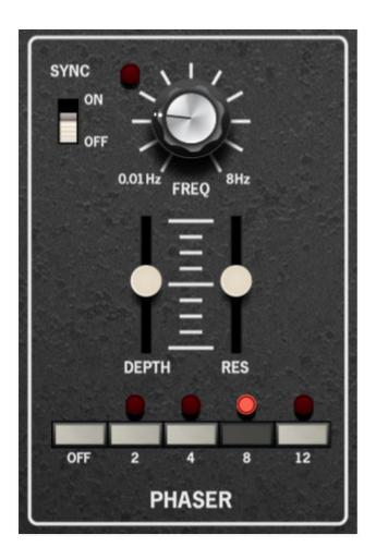
**Sync**- The *Sync* slide switch locks the rate of the Phaser's modulation LFO to the tempo in the top toolbar when using The Cat standalone version, or to the current project tempo when the plug-in version is used in a DAW. When engaged, the *Freq* knob snaps to note values ranging from 1/64th note triplet to 8 beats.
