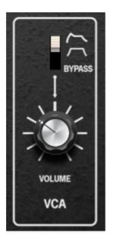
**Volume and modulation controls**- The VCA section controls overall amplitude (volume). The slides switch chooses between amplitude control via the ADSR envelope generator, the AR envelope generator, or *Bypass* mode.
