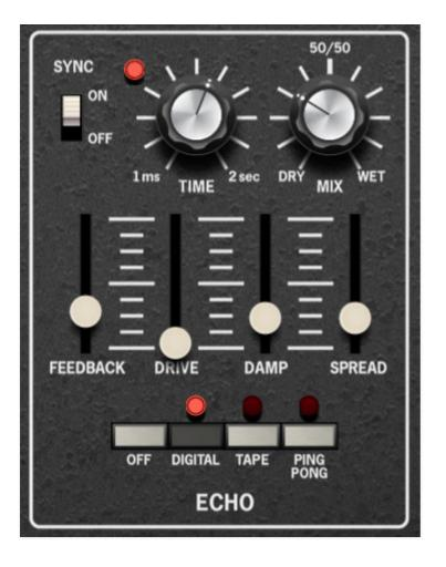
**Sync**- The *Sync* slide switch locks the delay time to master tempo. When engaged, the *Time* knob snaps to note values ranging from 1/64th note triplet to 8 beats. *Sync* mode locks to the tempo in the top toolbar when using The Cat standalone version or the current project tempo when the plug-in version is used in a DAW.
