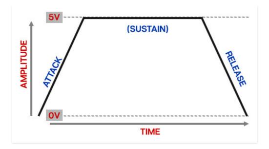
The attack stage defines how long it takes for the output voltage to rise from 0 to 5 volts. Once the attack stage reaches 5V, it remains there until the key is released. The release control defines the length of time it takes for the voltage to fall back to 0V when the gate input voltage is removed, i.e. when the key is released.
