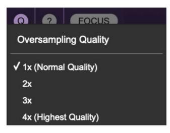
**Q Oversampling Quality -** The Q button sets Octave Cat's internal oversampling rate; the higher the setting, the better audio fidelity will be, with the caveat that more computer processing power will be required.
