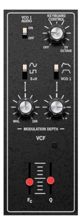
Cherry Audio's Cat filter is based upon the original four-pole 24 db/oct "cascaded OTA" SSM2040 filter. This filter was used in a number of 70s and 80s analog synths, including the original Rev 1 and Rev 2 Prophet-5.
